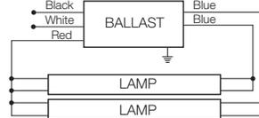
Note: For one lamp application, cap any blue lead. Insulate to 600 volts.
