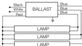
Note: For two lamp application, cap any blue lead. For one lamp application, cap any two blue leads. Insulate to 600 volts.
