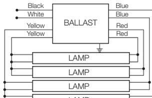
Note: For three lamp application, cap any unused blue lead. For two lamp application, cap two blue leads individually. For one lamp application, cap two blue leads, one red and one yellow lead individually. Insulate to 600 volts.
